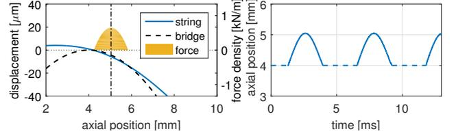
Figure 2: Left: string motion snapshot obtained with a model simulating distributed bridge contact [17]. The profile of the orange surface indicates force density, and the dash-dot line indicates the corresponding instantaneous central contact point. Right: Variation of the central contact point over the first 12ms. The flat dashed lines indicate periods of no contact.
