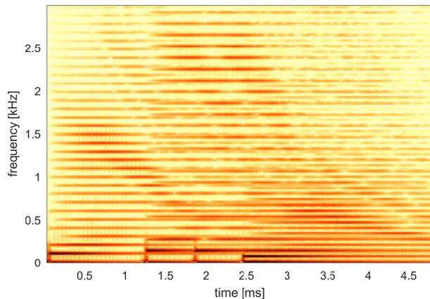
Figure 11: Spectrogram of a four-string tanpura bridge driving force signal. The strings were excited at  $t_e = 0, 1.2, 1.8,$  and  $2.4s$ , respectively.
